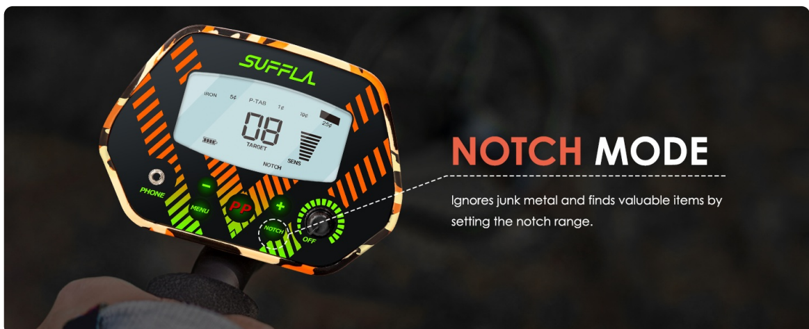
The LCD display in 'NOTCH MODE', illustrating how to ignore junk metal and find valuable items by setting a specific notch range.
