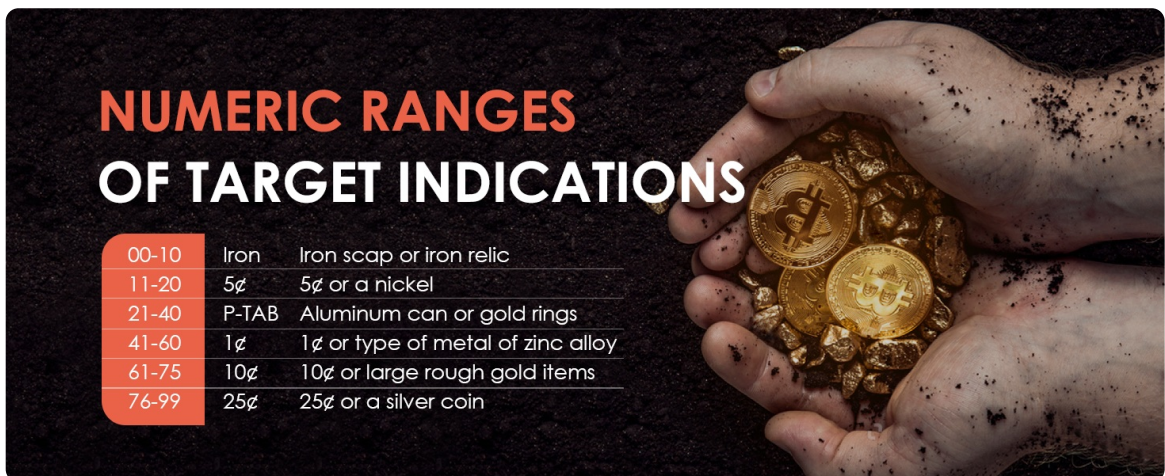
A visual representation of the numeric ranges displayed on the LCD screen, correlating to different types of metal targets.
