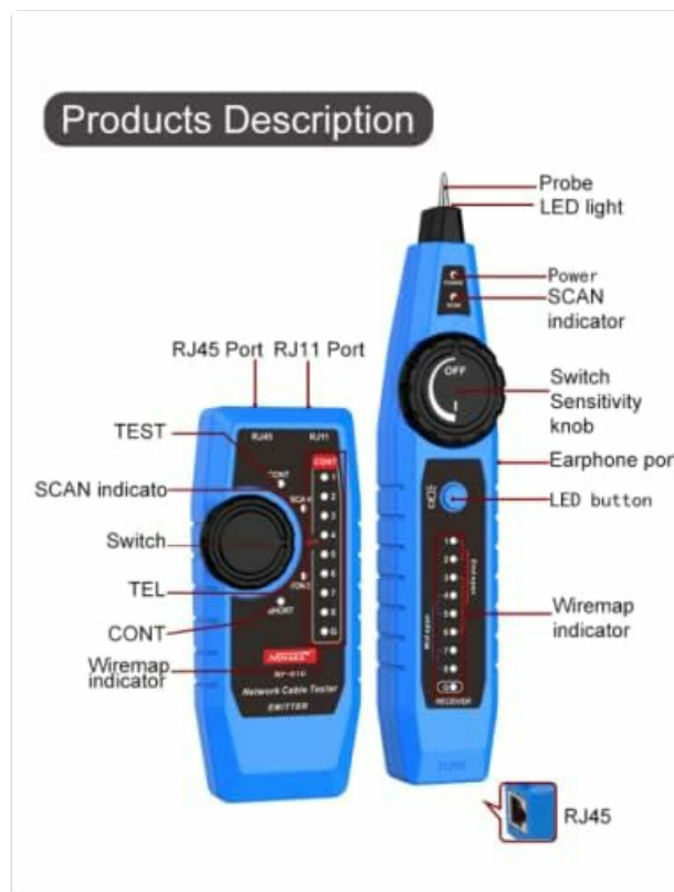
Figure 4.1: Labeled diagram of the NF-810 Emitter and Receiver units.
