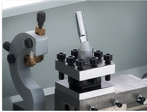
Figure 5.2: The adjustable tool post holds various cutting tools securely.
