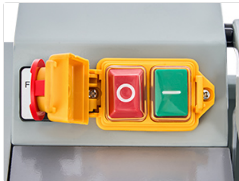
Figure 5.1: The main power switch (green) and emergency stop button (red) are located on the control panel.
