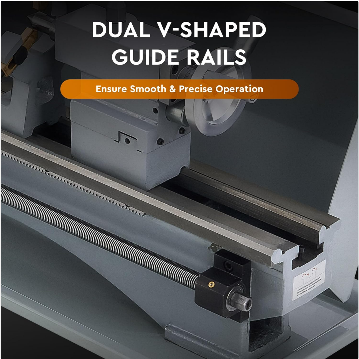
Figure 3.4: The dual V-shaped guide rails ensure smooth and precise movement of the carriage and tailstock.
