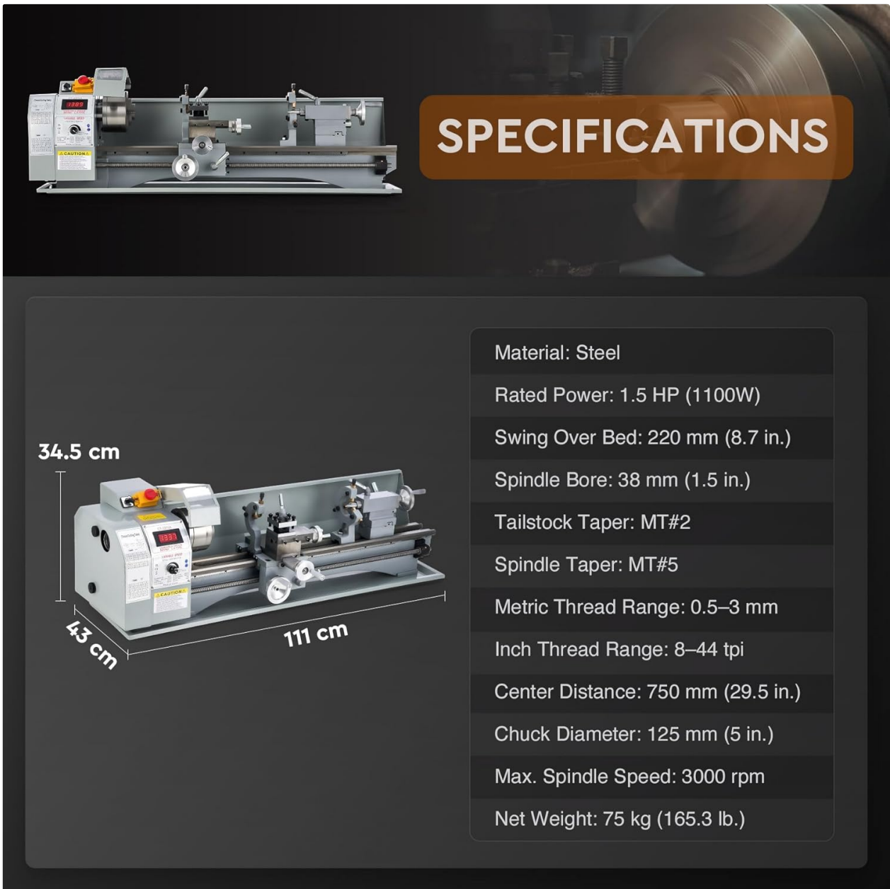
Figure 8.1: Visual representation of the lathe with key dimensions and specifications.
