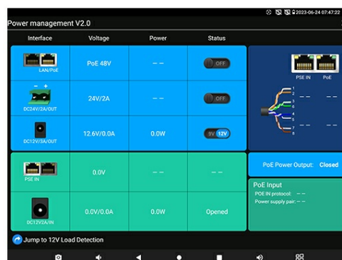
Figure 6.10.2: PoE Power Output and Power Management interfaces.
