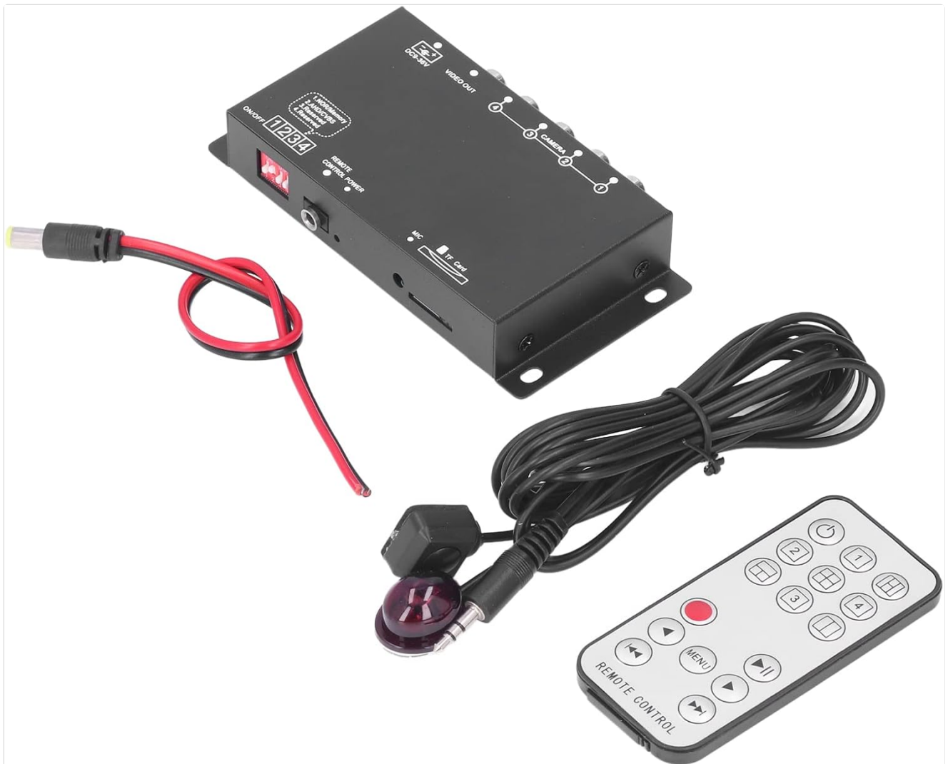
Image 7.1: The MDVR unit along with its accessories, including the remote control and power cable.
