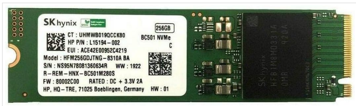
Figure 1: The SK hynix BC501 M.2 2280 NVMe SSD. This image shows the physical appearance of the SSD, highlighting its compact M.2 form factor, the NVMe interface connector, and the label displaying model information (HFM256GDJTNG), capacity (256GB), and brand (SK hynix).
