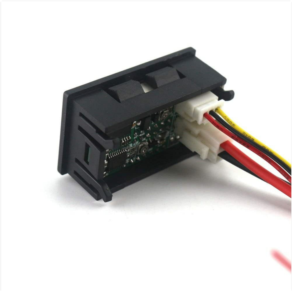
Figure 4.1: Rear view of the meter showing the wiring terminals. This image illustrates the connection points for the power supply, current input, and voltage measurement.
