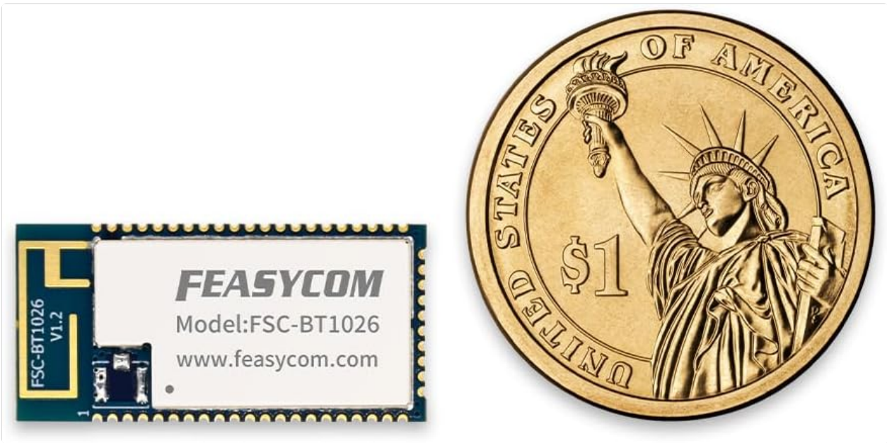
Image 6.2: The FSC-BT1026D module shown alongside a US dollar coin, illustrating its compact size.
