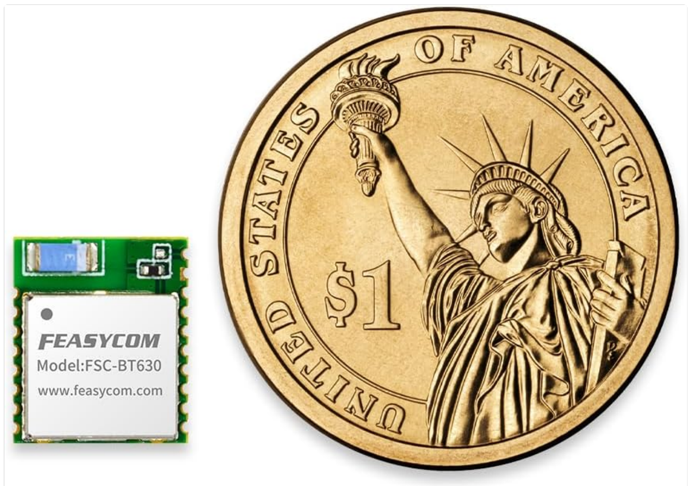
Figure 4.1: Size comparison of the FSC-BT630 module with a US dollar coin.
