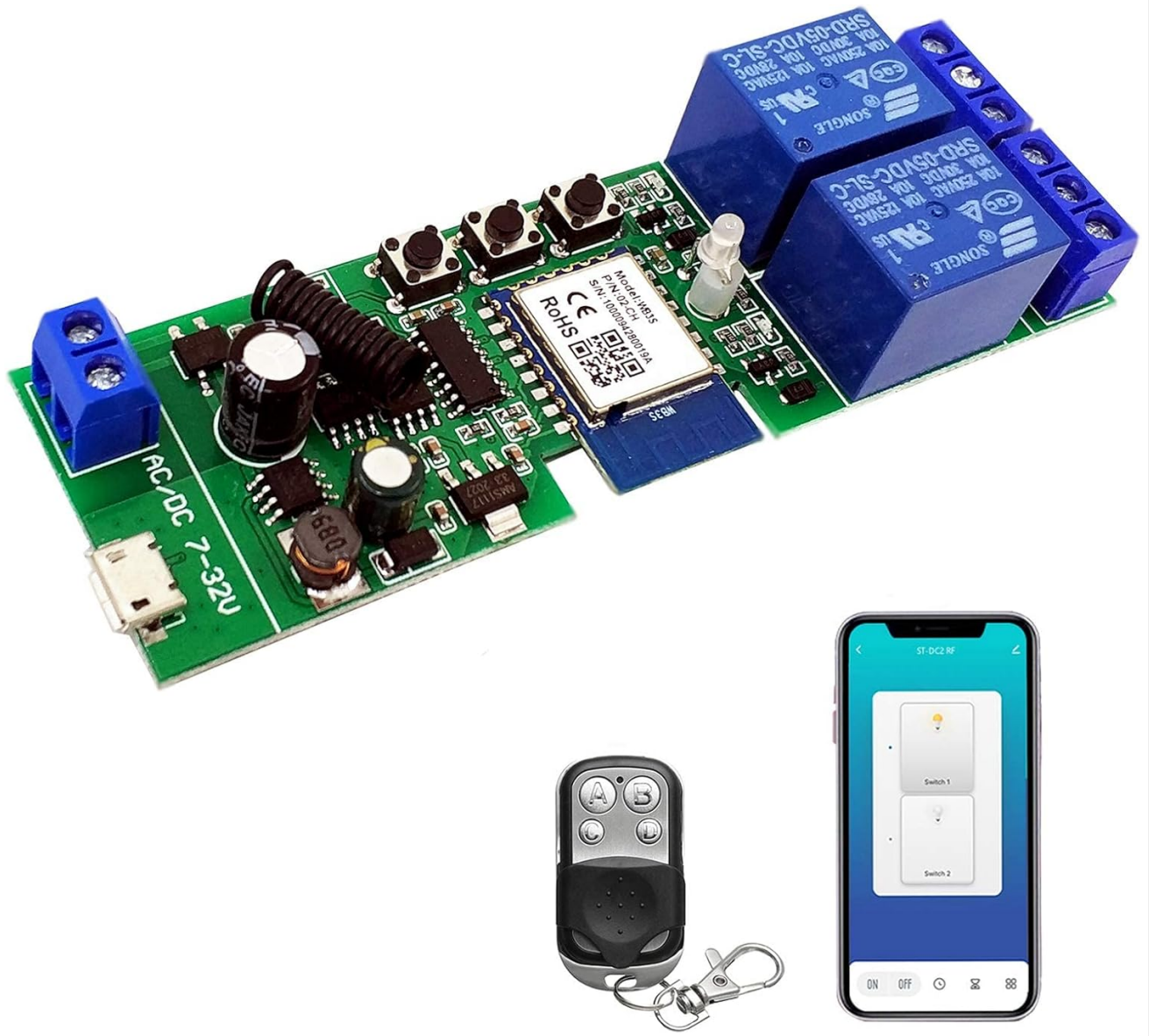
Figure 1: Newgoal 2-Channel WiFi Wireless Smart Switch module, accompanied by its 433MHz RF remote control and a smartphone displaying the Tuya/Smart Life app interface.
