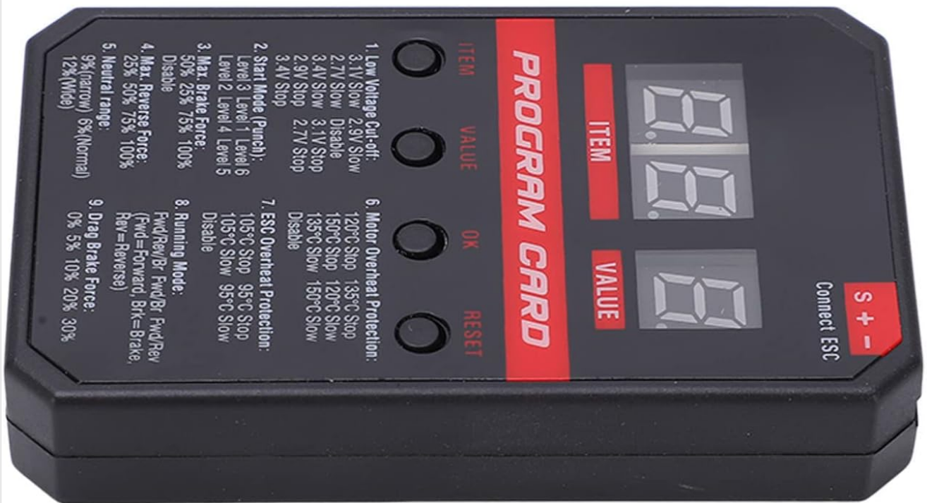
Image: A close-up view of the program card, highlighting the 'ITEM', 'VALUE', 'OK', and 'RESET' buttons, along with the digital display.
