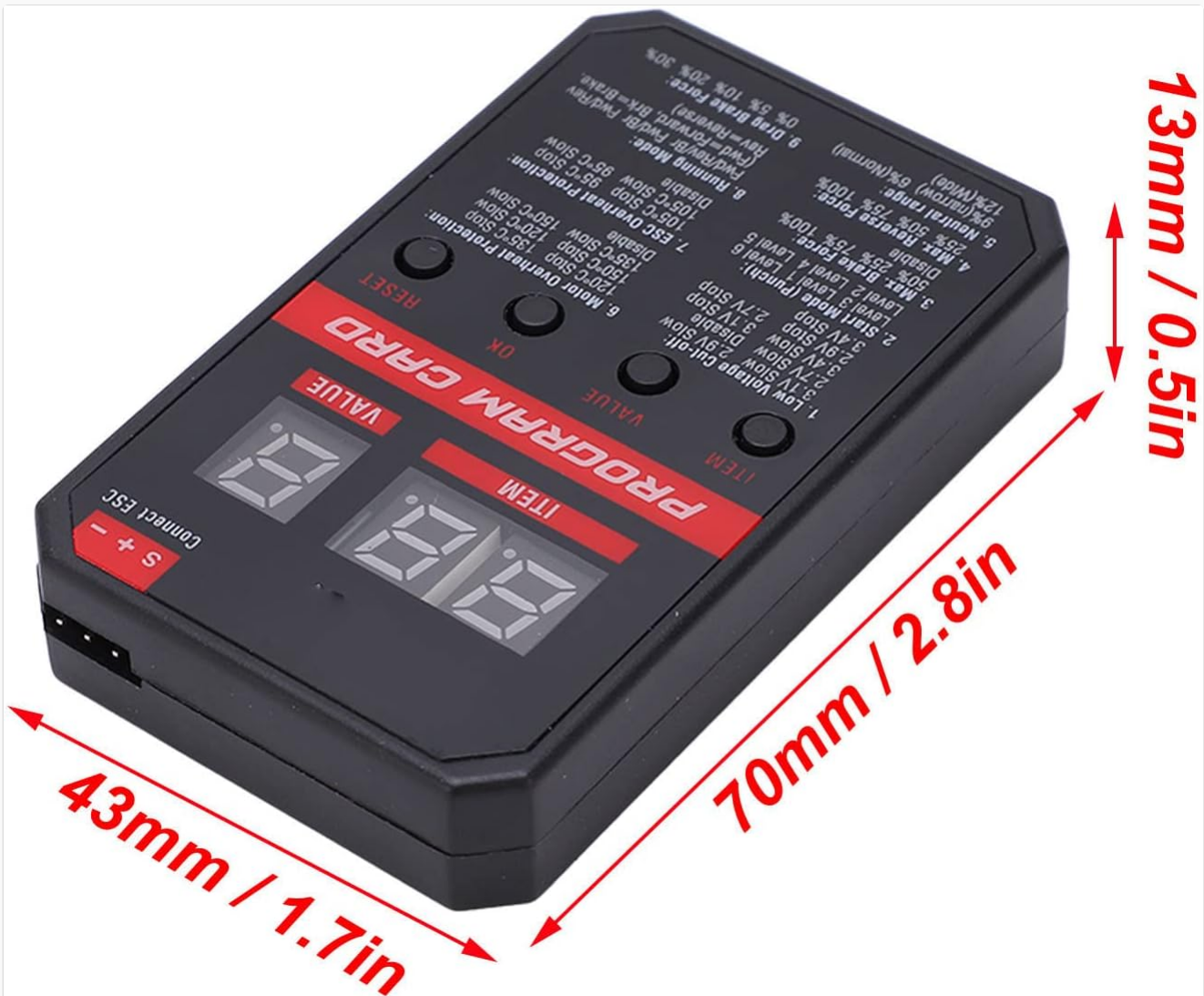
Image: The program card shown with its approximate length, width, and height measurements.
