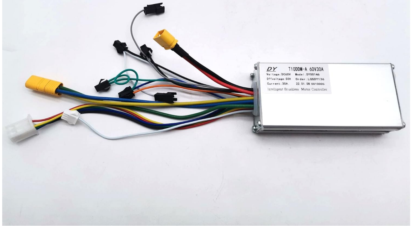
Figure 4.2: The controller with an overlay indicating its compatibility with Zero 10X scooters and its 60V operating voltage, confirming its intended application.
