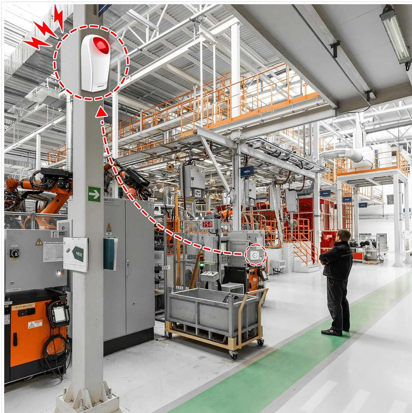
Image: An illustration of the siren's industrial application, where a call button in a factory setting wirelessly activates the siren located within the factory.
