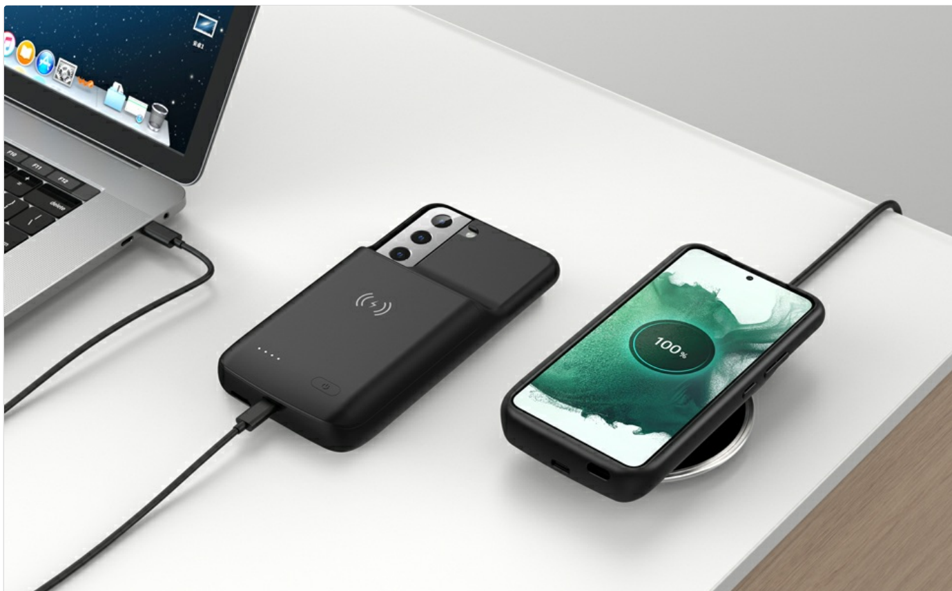
Image: This image displays the battery case simultaneously charging a phone and being recharged via a USB-C cable connected to a laptop.
