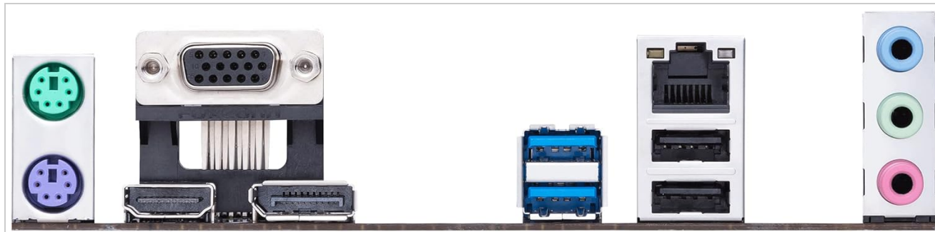
Figure 3: Rear I/O panel showing various connectivity ports including HDMI, DisplayPort, USB, and Ethernet.
