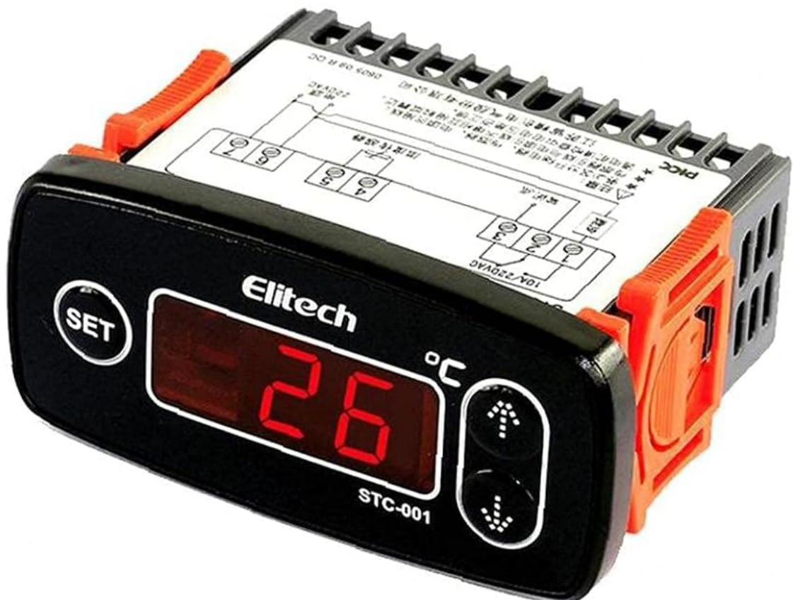
Figure 3: Image illustrating the primary functions of the Elitech STC-001, such as temperature control and alarm capabilities.
