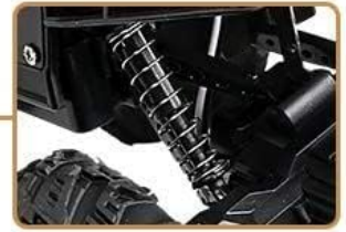
Independent shock absorption
