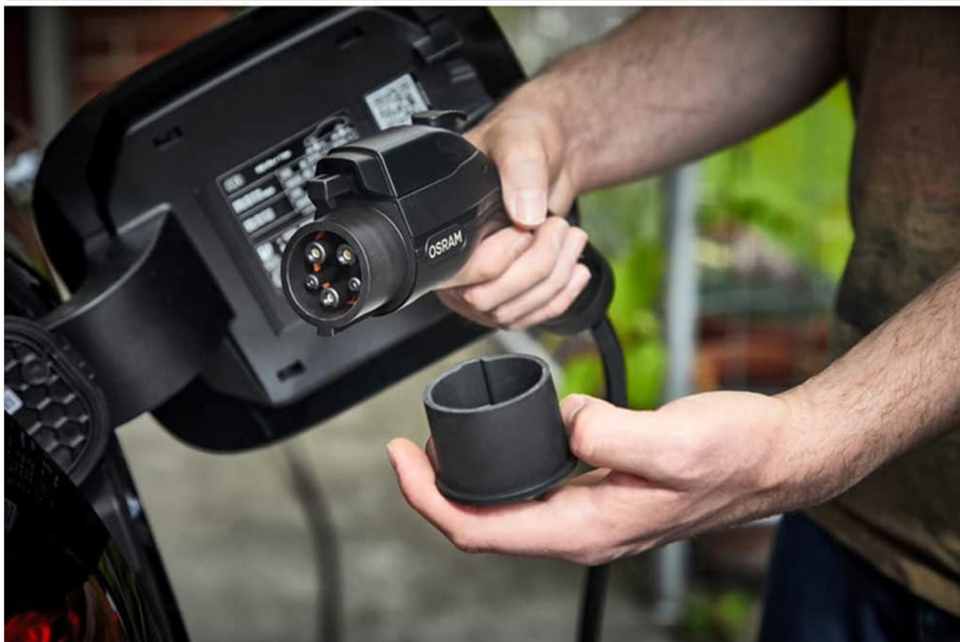
Image: A hand holds the Type 1 connector, preparing to insert it into the electric vehicle's charging port.
