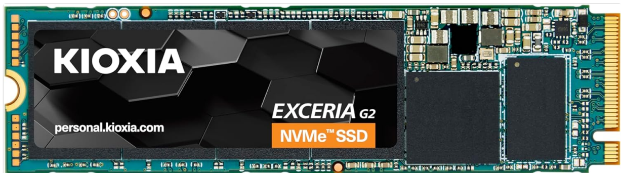
Figure 1.1: Top view of the KIOXIA EXCERIA G2 NVMe SSD. This image displays the compact M.2 2280 form factor with the KIOXIA branding and EXCERIA G2 NVMe SSD label clearly visible on the black heat spreader.
