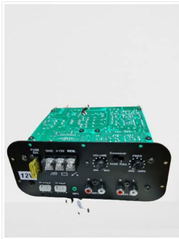
Figure 1: Front view of the Multisonic Amplifier Stereo MS-04. This image displays the main unit, showing the LED display, control knobs, and various input ports on the front panel.
