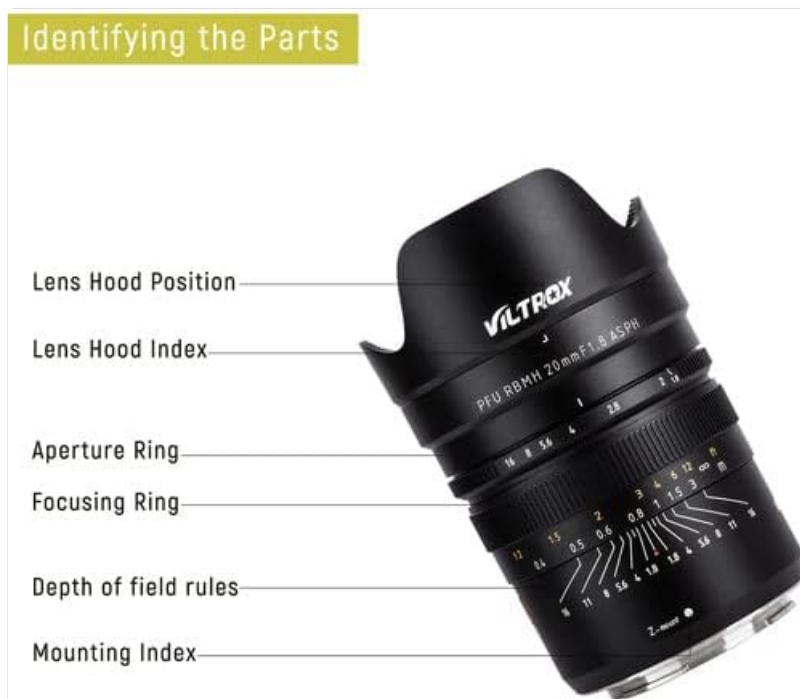
Figure 2.2: Key components of the Viltrox PFU RBMH 20mm f/1.8 ASPH lens.
