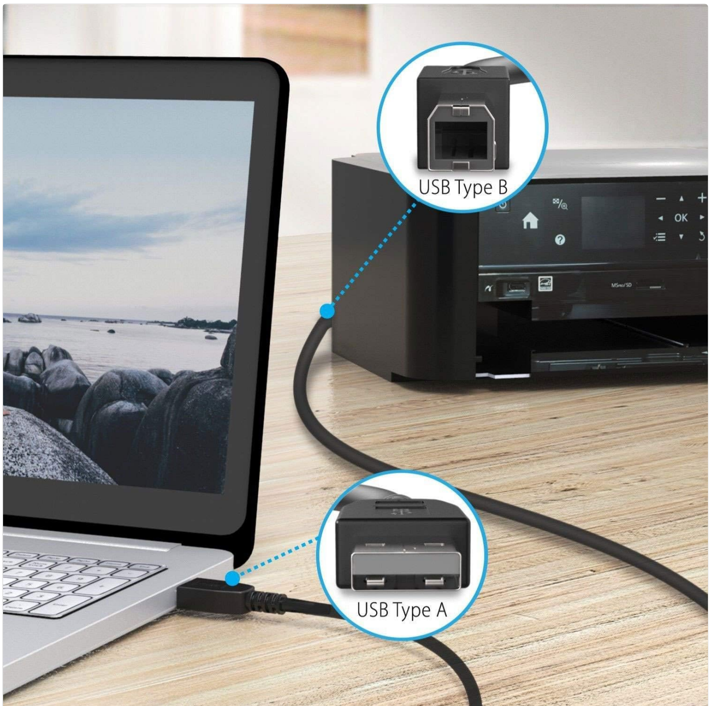
Image: An illustration demonstrating the connection of the USB Type-A end of the cable to a laptop and the USB Type-B end to a printer, with labels indicating the respective port types.
