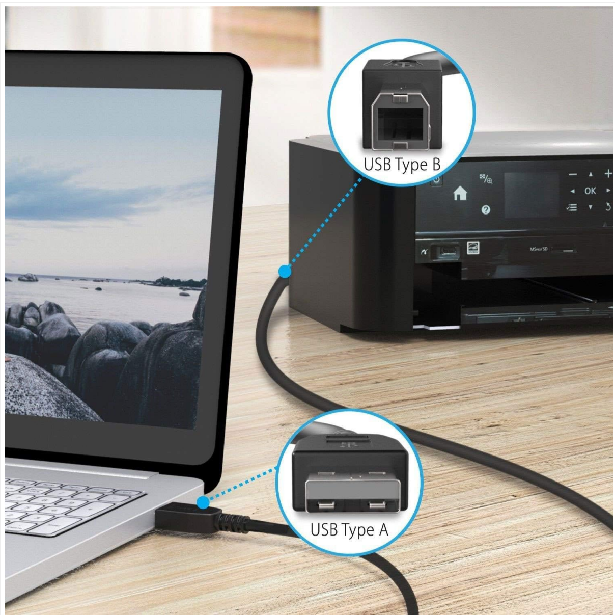
Figure 3: Illustration of connecting the USB Type-A end to a laptop and the USB Type-B end to a printer, demonstrating typical cable usage.
