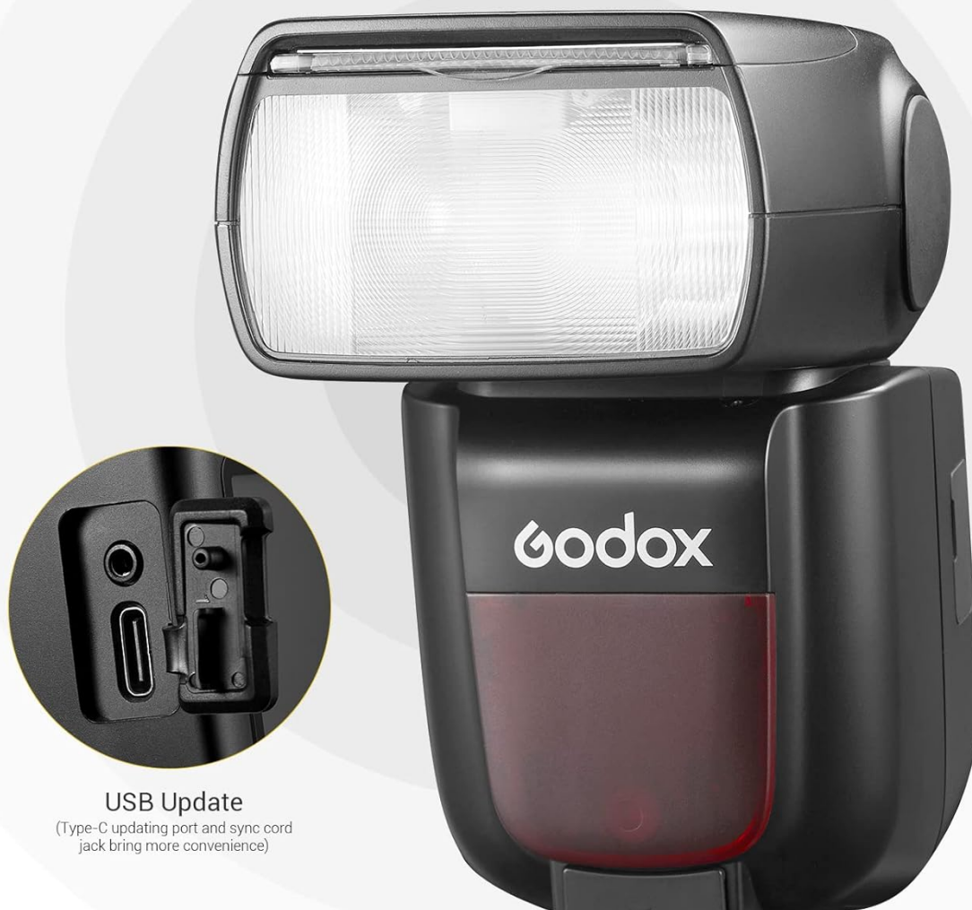
Image 5.1: The USB-C port for firmware updates and a sync cord jack, providing connectivity options.
