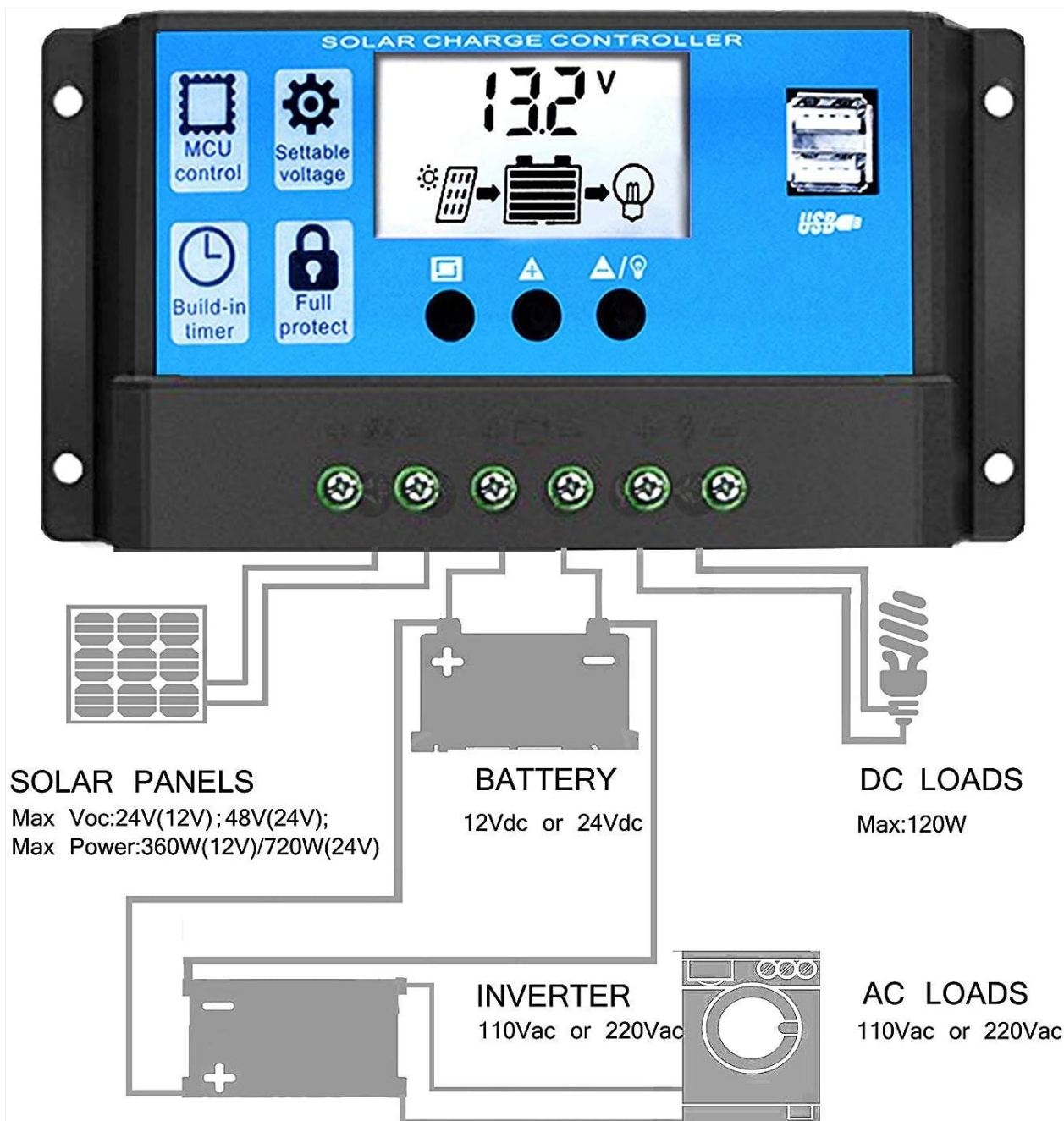
Image 5.1: Wiring diagram illustrating connections for solar panels, battery, DC loads, and optional AC loads via an inverter.
