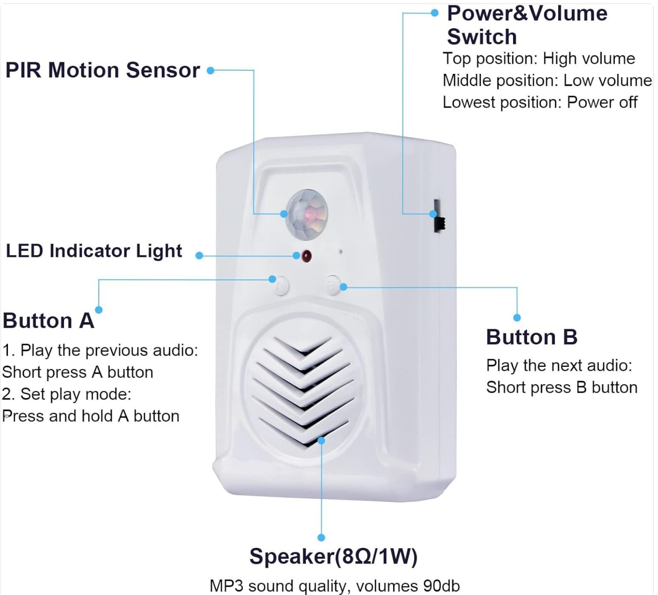
Image: Front view of the speaker with PIR Motion Sensor, LED Indicator Light, Button A, Button B, and Speaker (8Ω/1W) labeled. The Power & Volume Switch is on the side.
