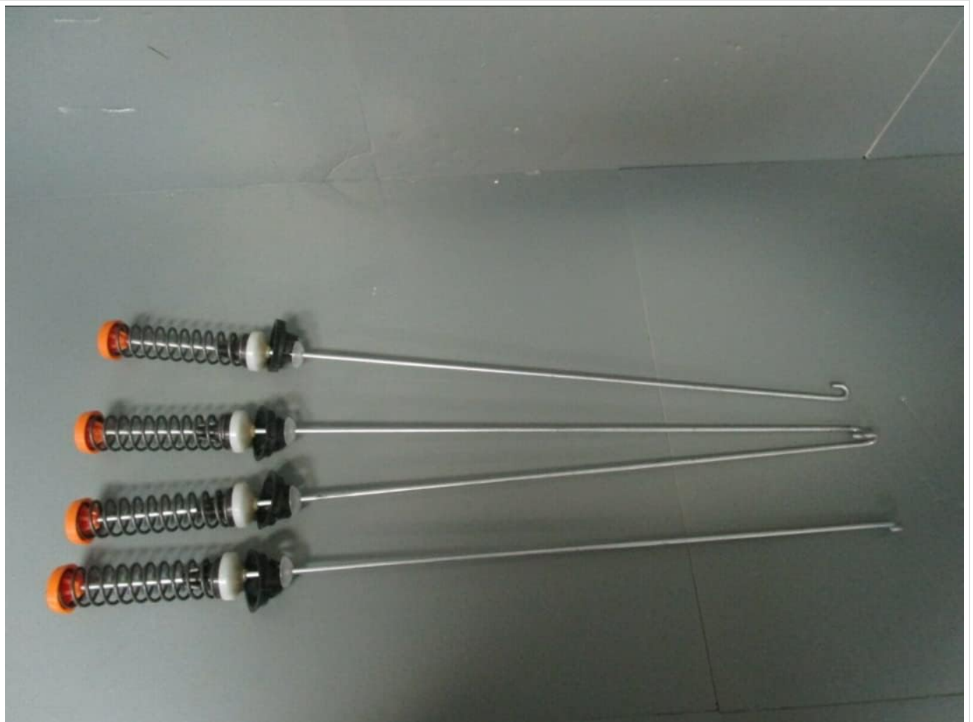
Image: Four new suspension rods, each featuring a metal rod, a spring, a white plastic ball joint, and an orange plastic cap. These
