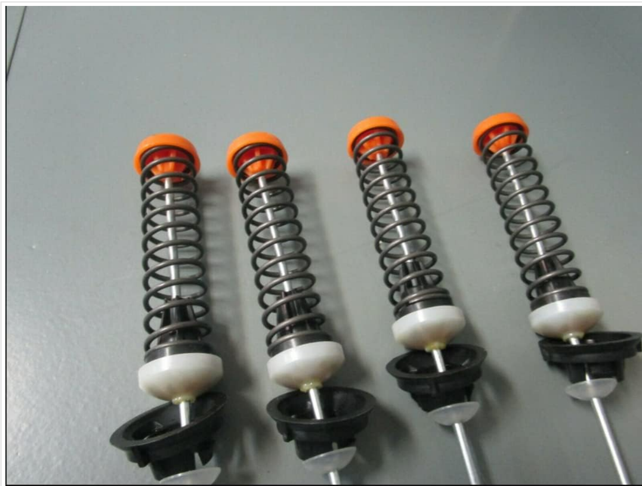
Image: A detailed view of the upper portion of a suspension rod, showing the coiled spring, the white plastic ball joint, and the orange plastic cap that sits atop the spring. This assembly helps absorb vibrations.
