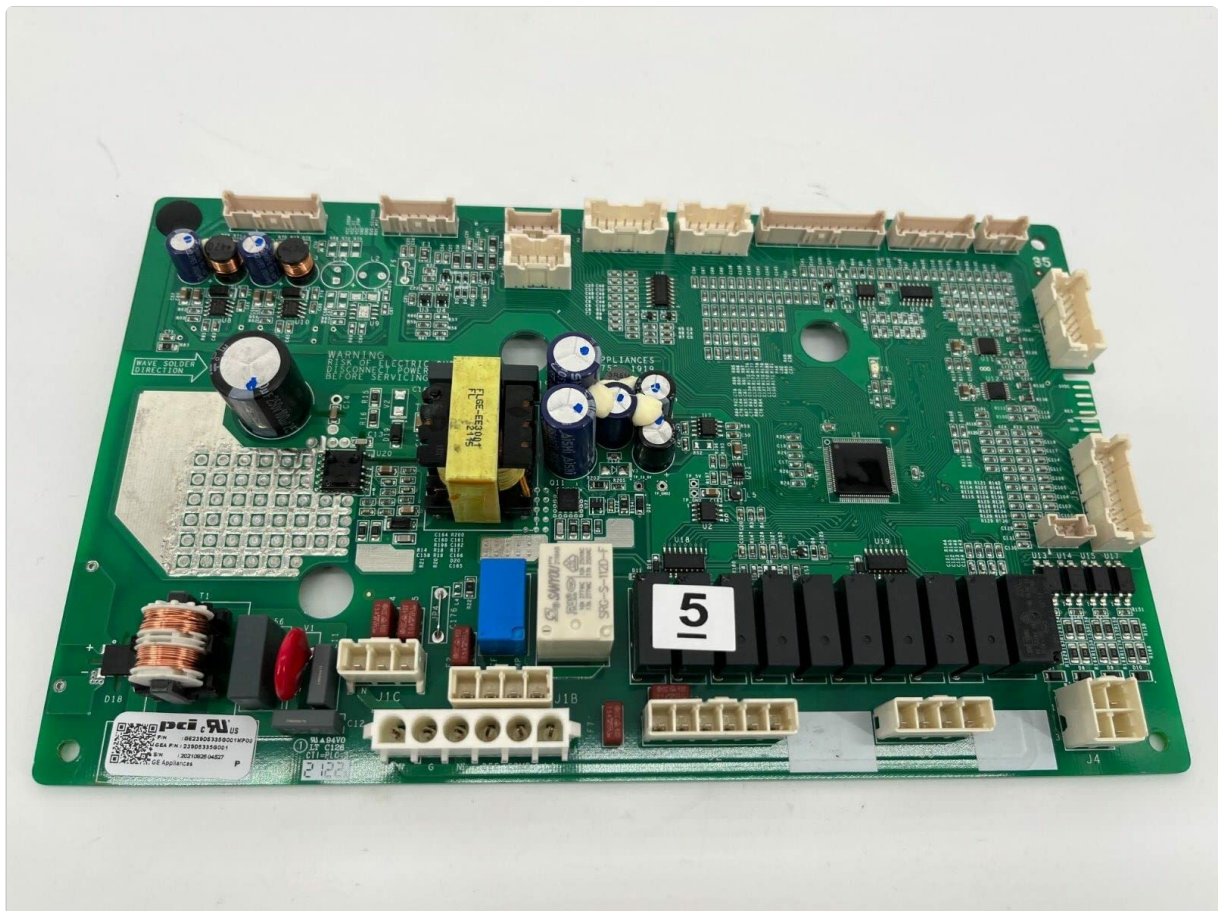
Image: The GE Refrigerator Main Control Board, model WR55X38248. This image shows the general appearance of the control board with various connectors and electronic components.
