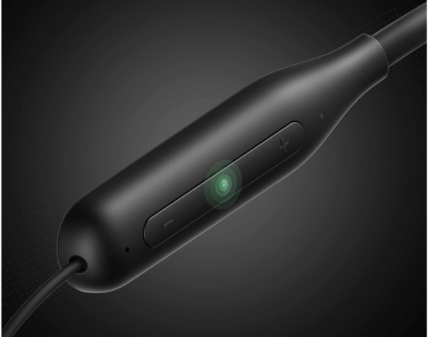
Image 3.2: Close-up view of the three control buttons on the neckband for managing audio and calls.
