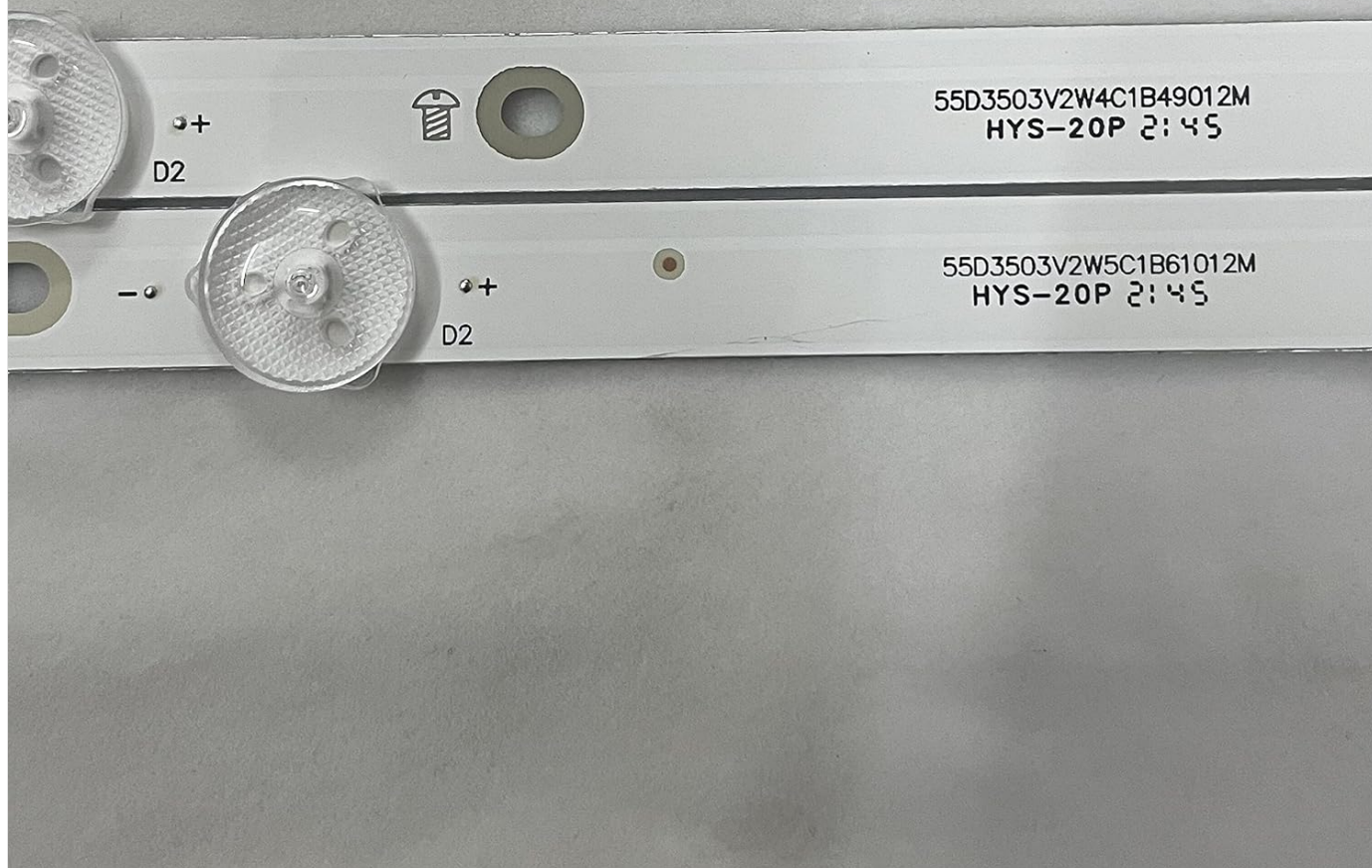
Figure 4.3: Additional markings such as 55D3503V2W4C1B49012M and HYS-20P for further identification.
