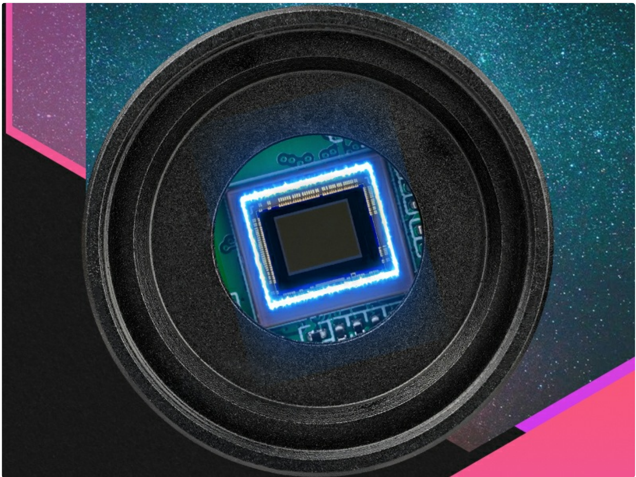
Figure 3: Close-up view of the SV905C's 1.23MP CMOS sensor.
