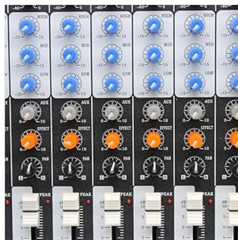
Figure 3: Detailed view of individual channel controls, including GAIN, 3-band EQ (High, Mid, Low), AUX, EFFECT, and PAN knobs.
