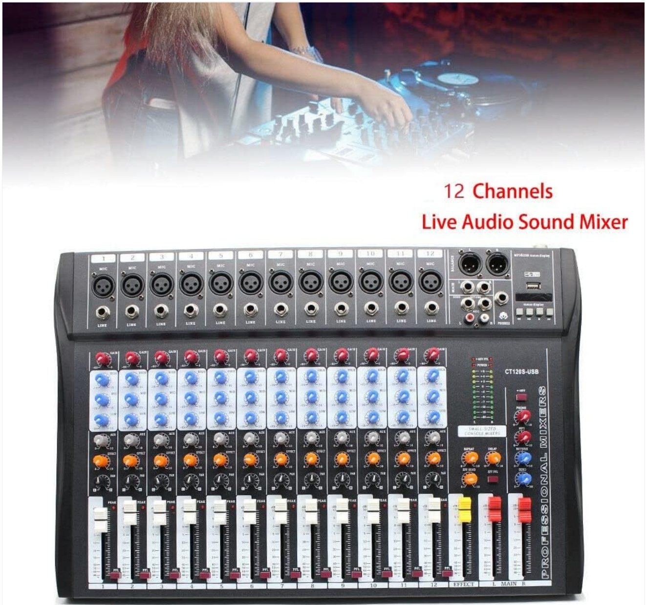
Figure 1: Front view of the TFCFL CT120S-USB 12 Channel Live Studio Audio Mixer, highlighting its 12-channel capability.
