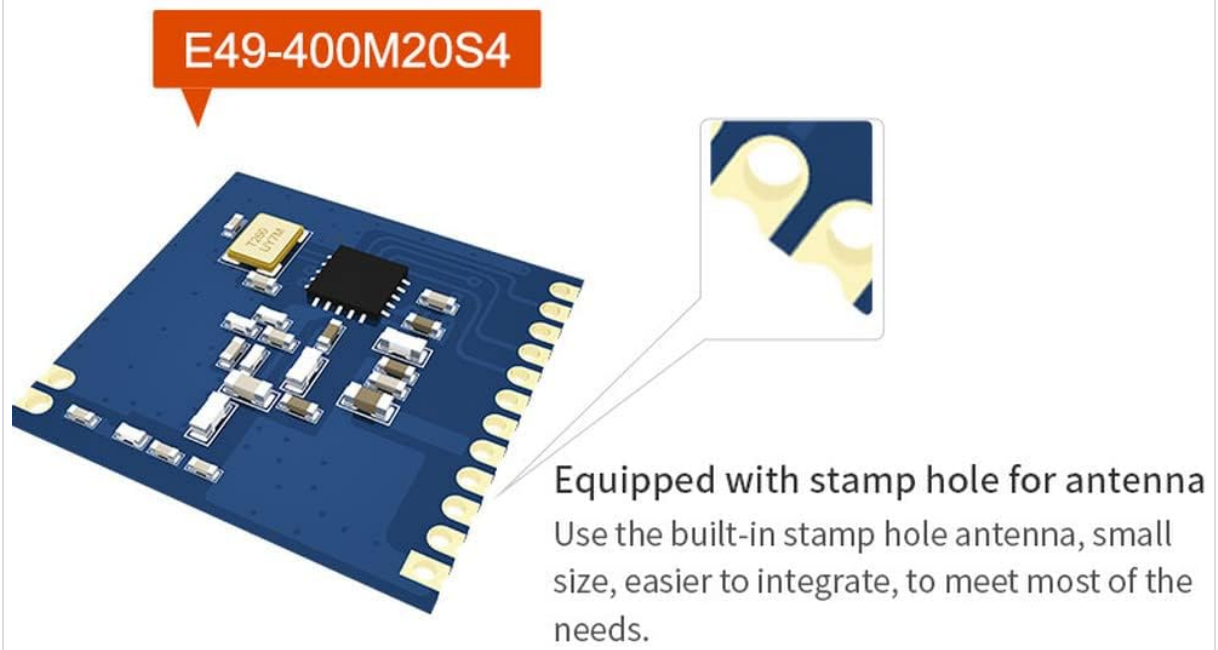
Figure 3: E49-400M20S4 Antenna Type. The module features a stamp hole for integrating an external antenna, adapting to various development needs.
