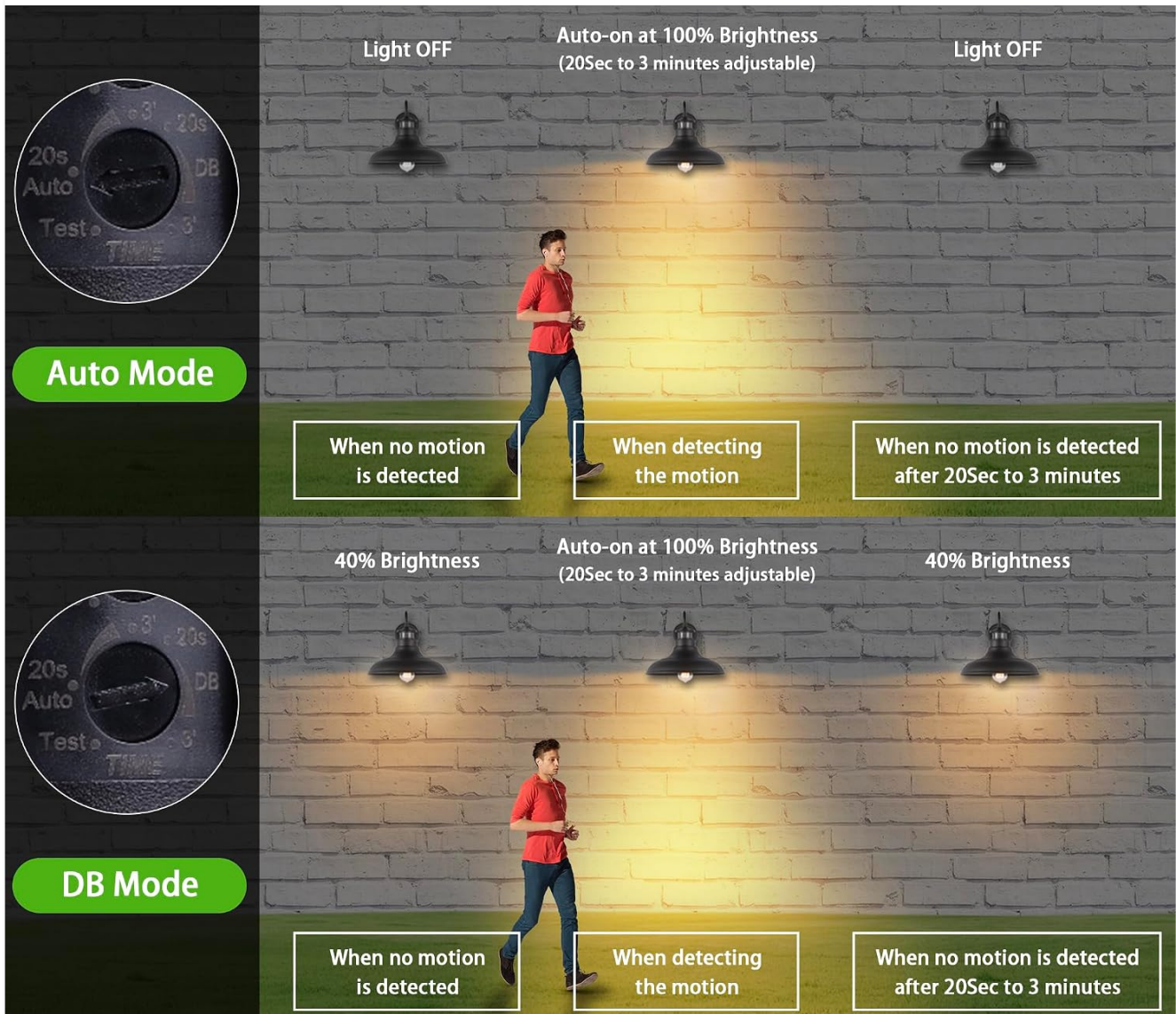
Image 6.1: Visual representation of DB Mode and Auto Mode operation, showing light behavior with and without motion detection.
