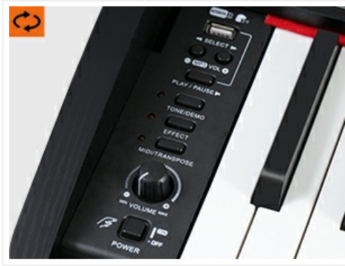
Image 6.1: A detailed view of the control panel, showing the power button, volume knob, and various function buttons for tone selection, effects, and MIDI/transpose.
