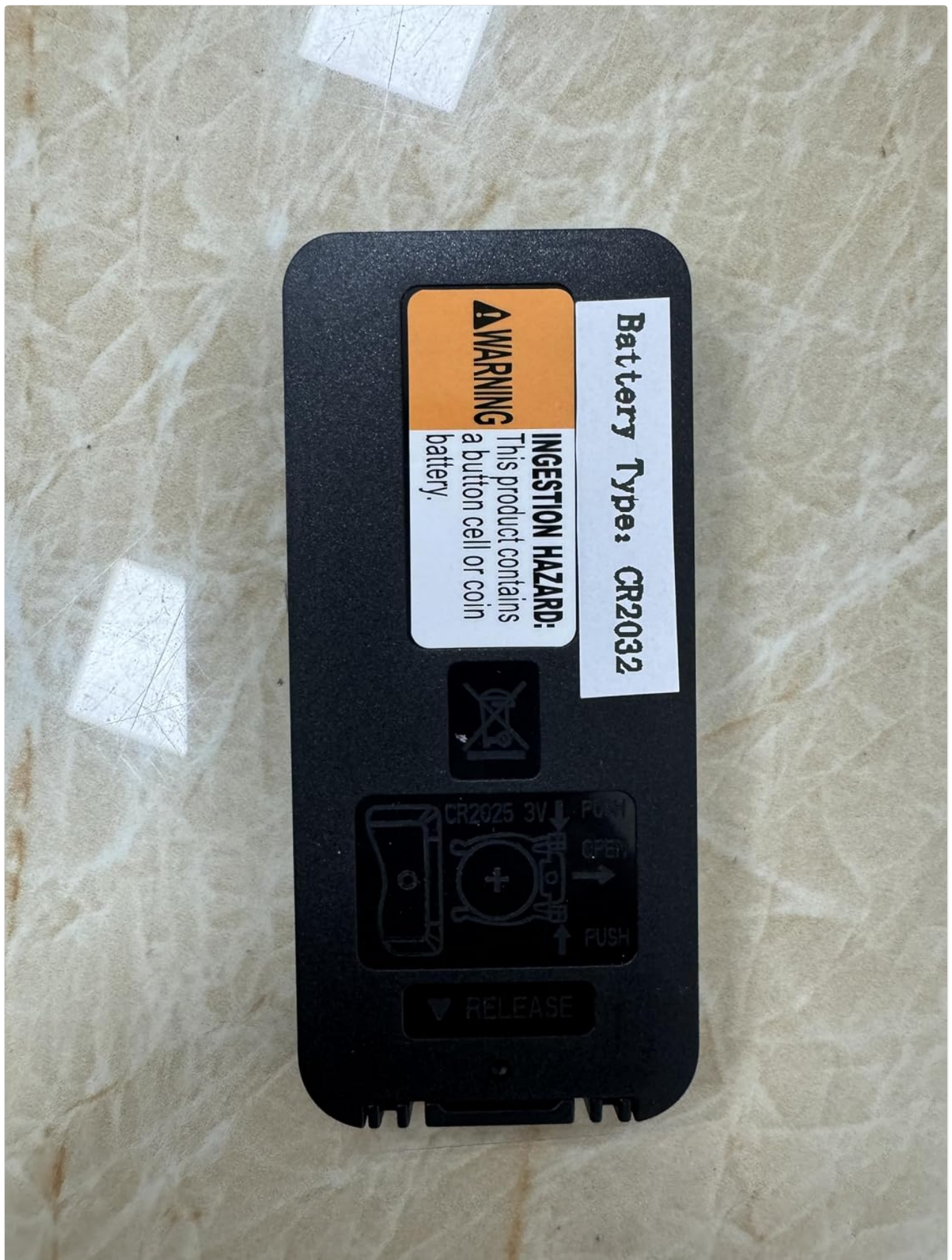
This image shows the battery compartment of the remote control, indicating the CR2032 battery type and a warning regarding ingestion hazard.
