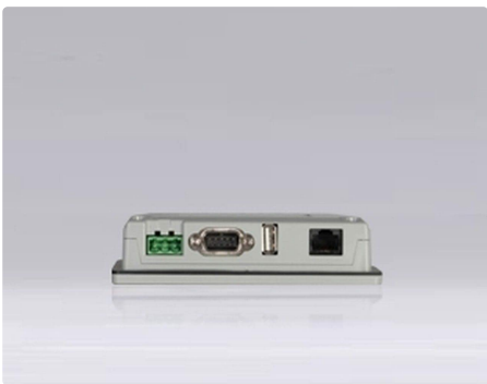
Figure 8.2: Top view of the MT6071iE HMI, highlighting the various communication ports including serial ports (DB9 connector), USB ports, and power input terminals. This view demonstrates the connectivity options available.
