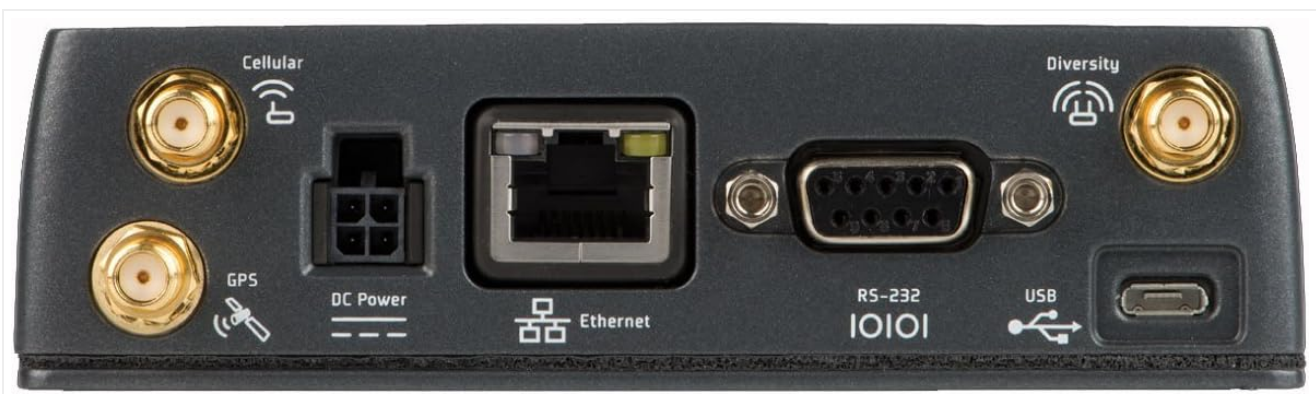
Image 2: Rear view of the Sierra Wireless AirLink RV50X router. From left to right, ports include: two Cellular antenna connectors, a GPS antenna connector, a DC Power input, an Ethernet port, an RS-232 serial port, and a USB port. A Diversity antenna connector is also visible on the far right.
