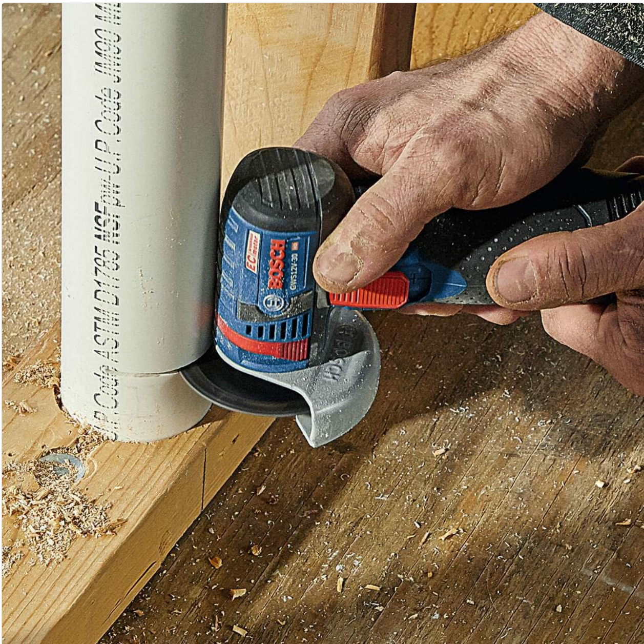
Figure 5: The Bosch CMW300 multi-wheel in action, cutting a PVC pipe, demonstrating its clean and efficient performance on plastic materials.
