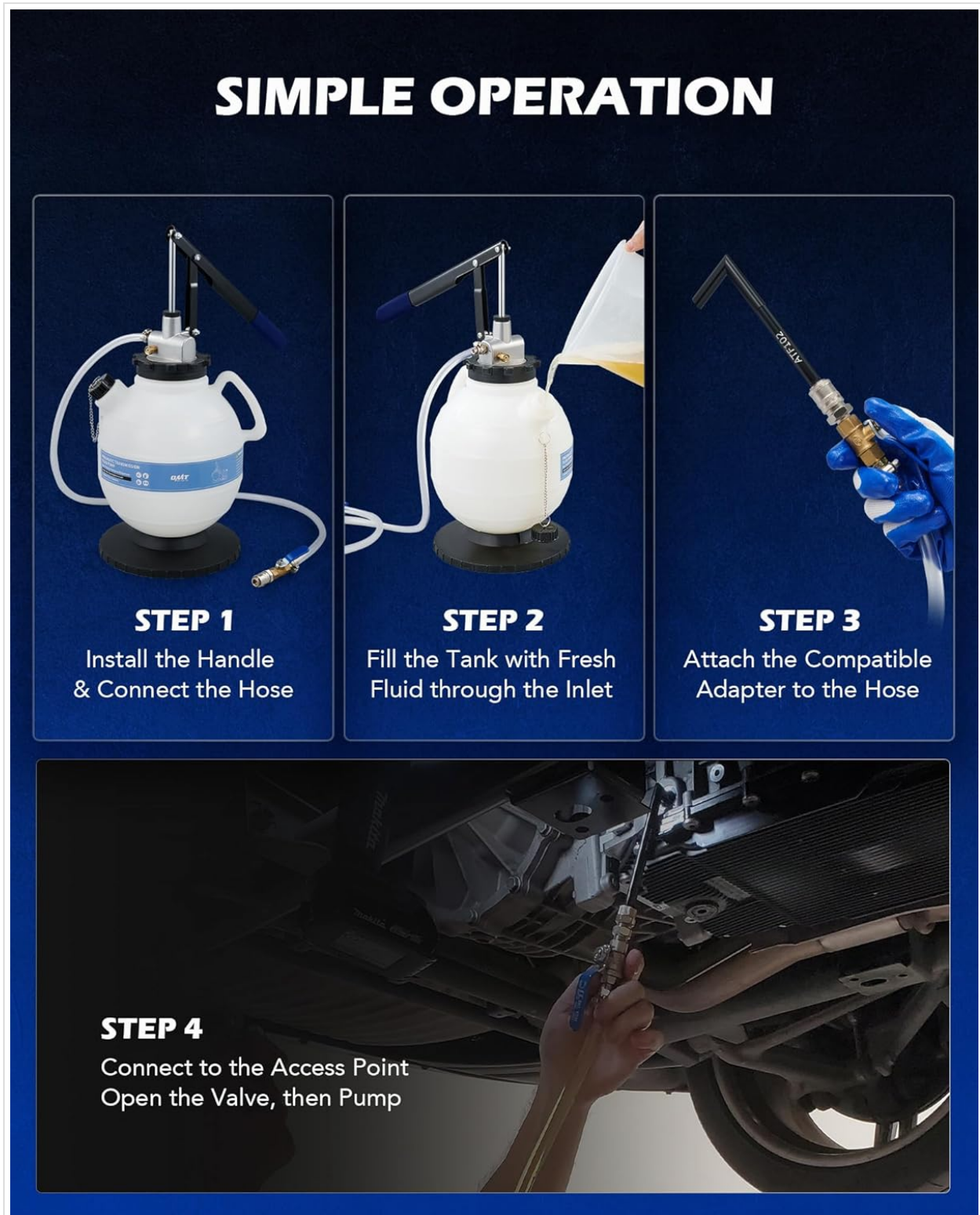
Figure 5: Step-by-step guide for operating the transmission fluid pump.
