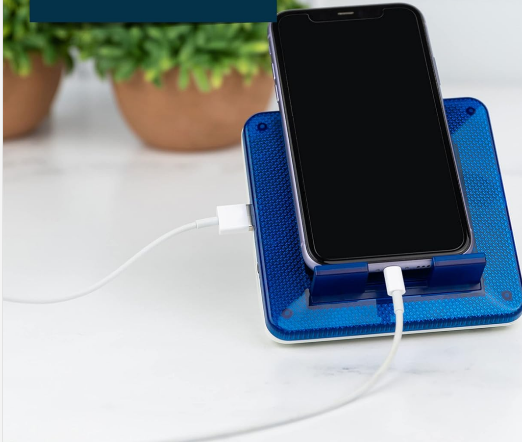
Image 4.1: Placing a smartphone on the RF-200 dock and connecting a charging cable.
