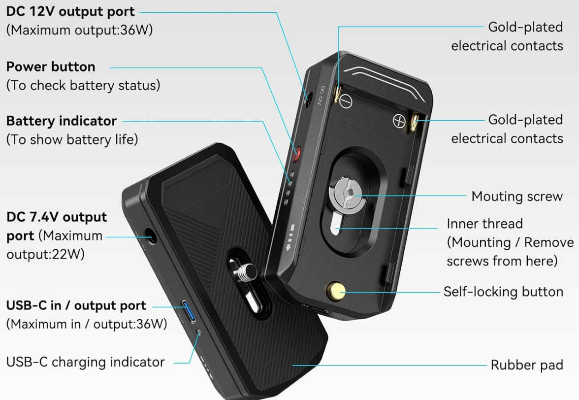
Image: Detailed diagram of the battery plate's components.
