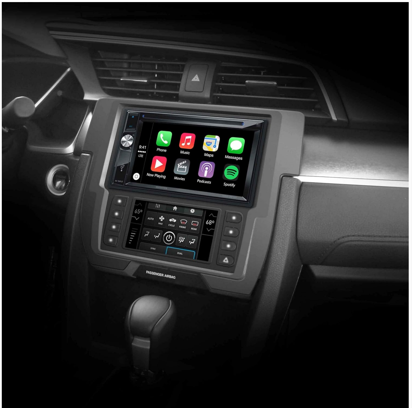
Image 4.3: The Metra 99-7821B dash kit shown installed in a Honda Civic dashboard, featuring an aftermarket double-DIN radio. This image demonstrates the integrated appearance of the kit within the vehicle's interior.
