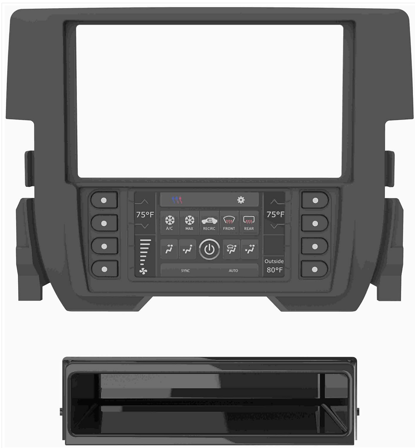
Image 4.1: Front view of the Metra 99-7821B dash kit, showing the integrated touchscreen and the opening for the aftermarket radio. The lower section includes a removable storage pocket for single-DIN radio installations.
