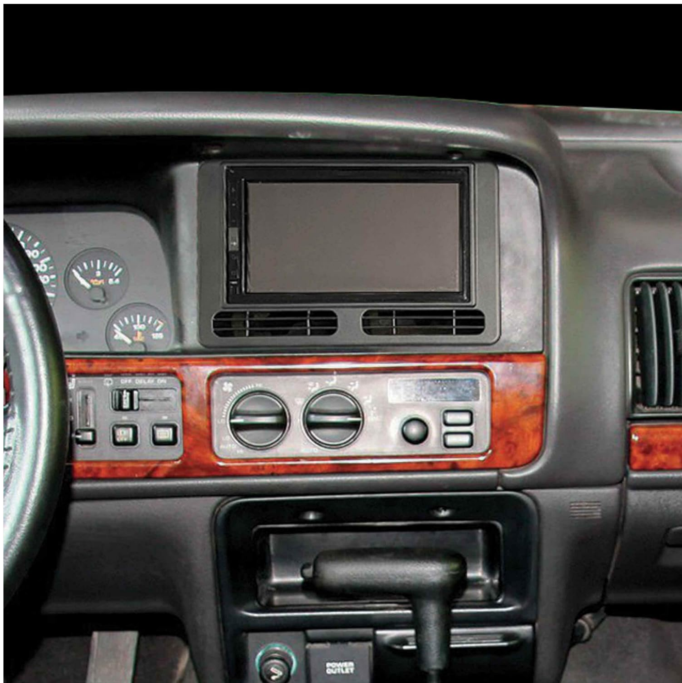
Image 4: Example of the Metra 107-CH5 kit installed in a 1996-1998 Jeep Grand Cherokee dashboard with an aftermarket radio.
