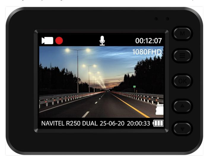
The screen of the Navitel R250 DUAL NV dash cam is shown, displaying a live road view with overlayed information such as recording status, microphone status, current time, video resolution (1080FHD), and battery level. A memory card icon is also visible.
