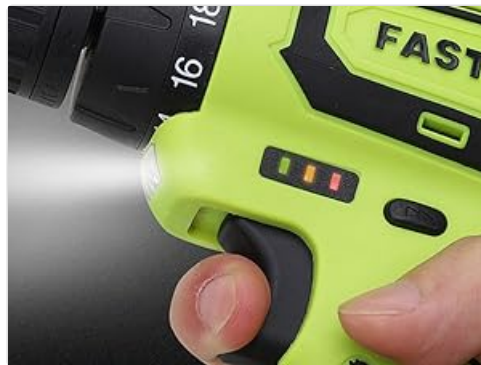
Image 4.1: Battery indicator lights on the drill driver.
