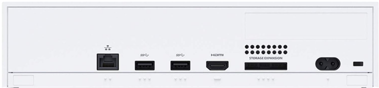
Image: The rear of the Xbox Series S console displays its various ports, including Ethernet, USB, HDMI OUT, storage expansion slot, and power input, for connecting peripherals and power.
