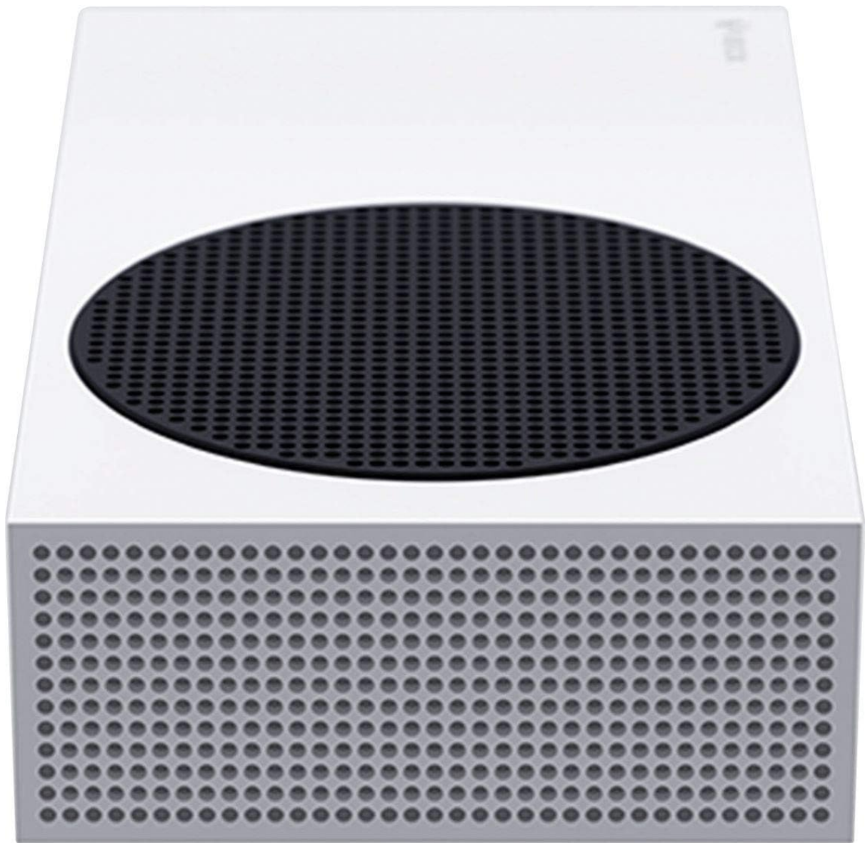
Image: A top-down view of the Xbox Series S console, highlighting the large circular black fan grille, which is a primary exhaust point for heat.
