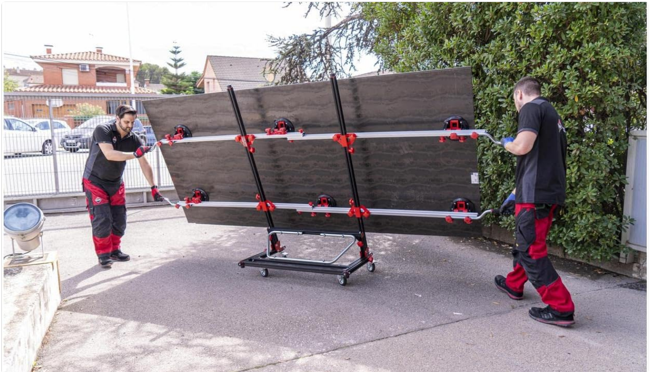
Figure 7: Two operators lifting a large slab using the Slim Easy Trans Plus.
