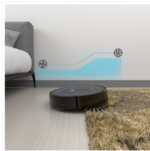
Image: The robot vacuum demonstrating its carpet boost feature, increasing suction power when moving from a hard floor to a carpeted area.
