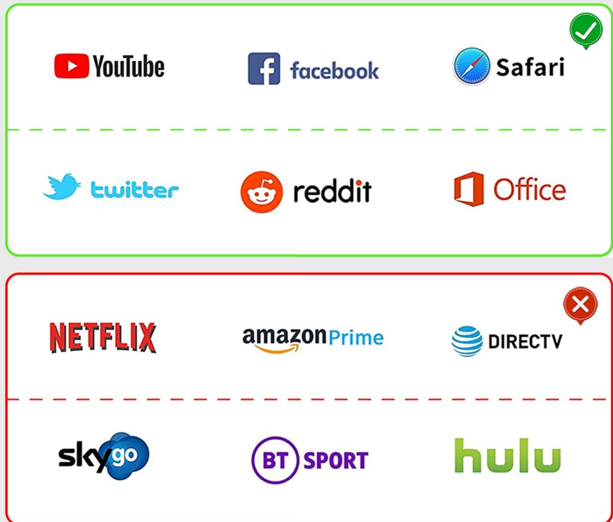
Figure 7: Chart indicating supported and unsupported streaming applications due to HDCP protection.
